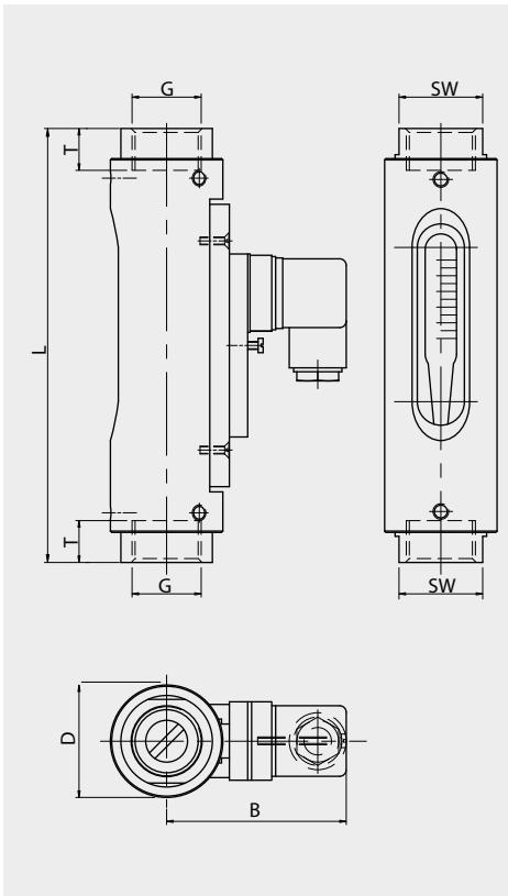
The technical drawings provide three views of the DUG flow monitor: a front view showing the threaded connection and glass window; a side view showing the height and mounting flange dimensions; and a cross-sectional view showing the internal float mechanism and measurement tube.
