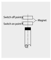
The extent of the switching hysteresis (stroke of the actuating magnet) is dependent on the size of the actuating magnet and the magnetic shunt via the iron content of the surroundigs. In the case of most magnetic switches it amounts to approximately 2 to 5mm stroke of the actuating magnet.
